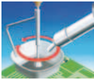
Desoldering IC component with hot air
